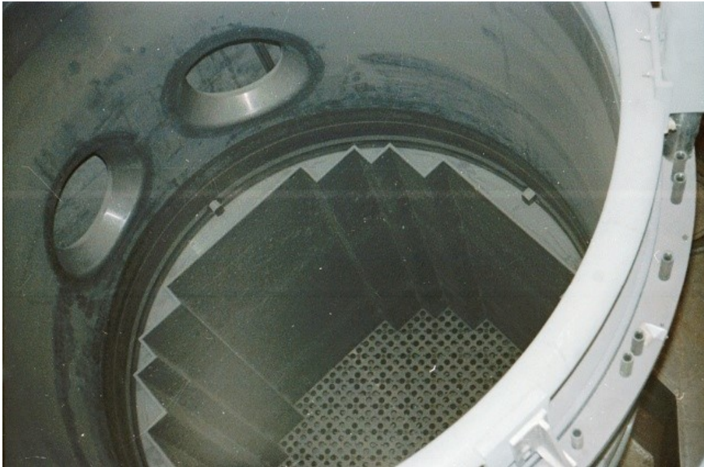
Looking down into the upper core barrel and core baffle and former assembly of a pressurized water reactor.
