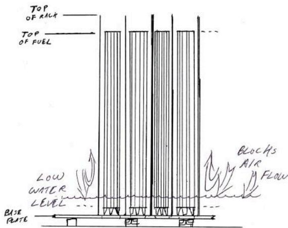
**Water addition:** adding water to the bottom of an empty spent fuel pool can damage an assembly with a heat rate of 7kw or less that has reached equilibrium in air! -- *The water can block the circulation of air and cause the fuel assembly to overheat. The heat removed by the low level of water is insufficient to cool the assembly.*
