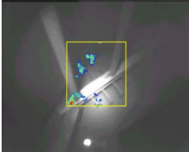
Figure 12. Image of the Bottom of Tank 8D-2 with a Gamma Camera 96
