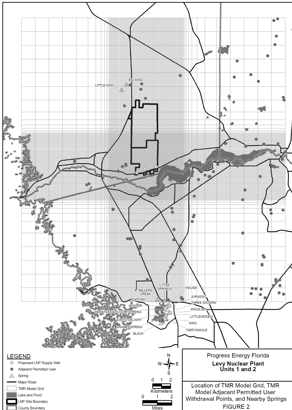
Figure 2-12. Local-Scale Model Grid Showing the Location of Proposed LNP Supply Wells, Adjacent Permitted Users, and Springs (PEF 2010)
