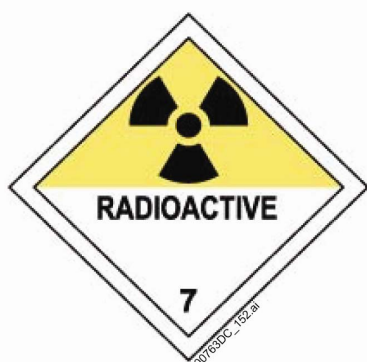
Figure H-2. Radioactive hazard communication placard.
