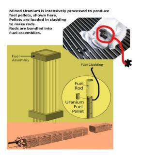
Note: Only fresh uranium can be held unshielded; after use (fissioning) in the reactor, irradiated fuel pellets give off a *lethal* dose of radiation in seconds. This waste must be shielded and handled robotically. Also thermally hot, it is cooled in pools by circulating water for years before it can be stored in dry containers.
