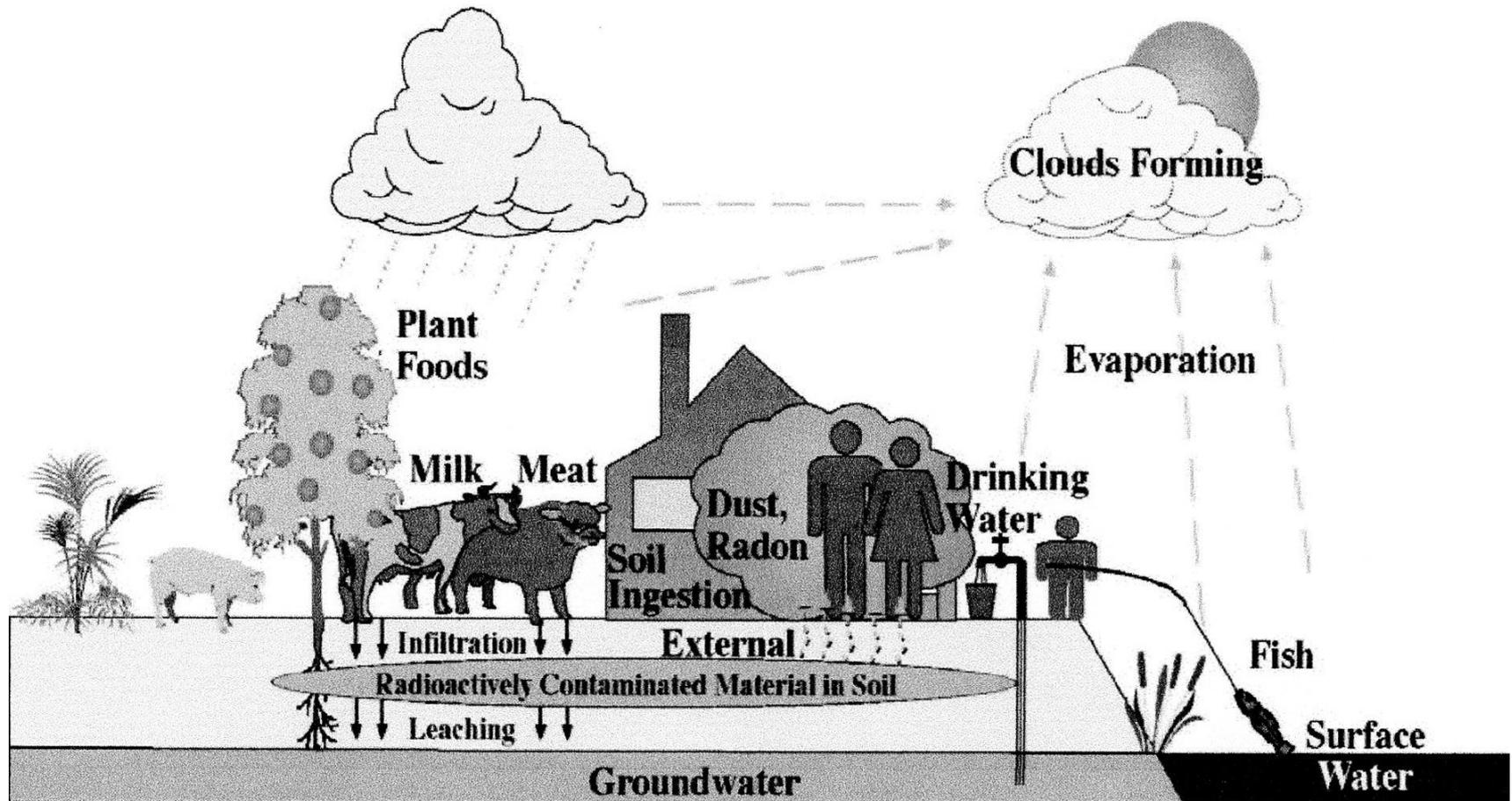
**RESRAD is a computer model designed to estimate radiation doses and risks from RESidual RADIOactive materials.**
