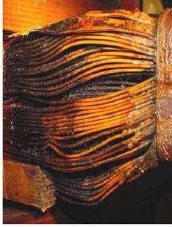
Courtesy Eskom, Makhosi, T., G. Coetzee Damaged Winding and Core on Eskom Transformers in South Africa
