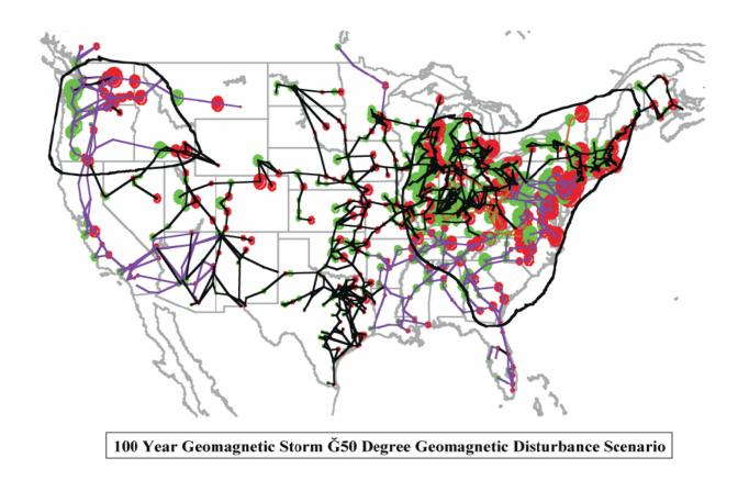
Figure 11: The simulation results showing the pattern of GIC flows in the U.S, grid for a 4800 nT/min geomagnetic field disturbance at 50 degrees geomagnetic latitude. The above regions outlined are susceptible to system collapse due to the effects of the GIC.
