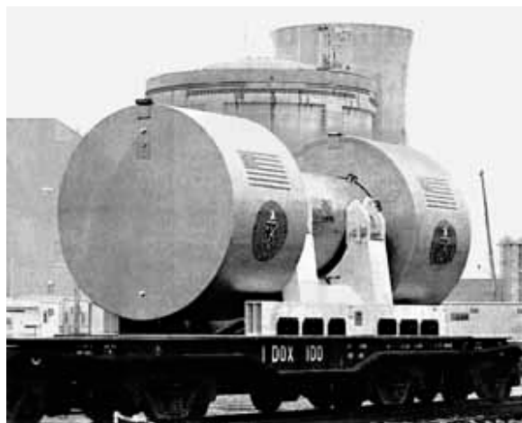
Radioactive waste rail shipping container (small). Reactor in background
