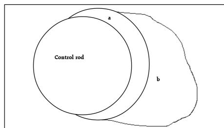
Comparison of Beznau-1 and Davis-Besse "holes". In Beznau-1, area a was corroded; in Davis Besse corrosion went deeper and further, reaching area b as well.
